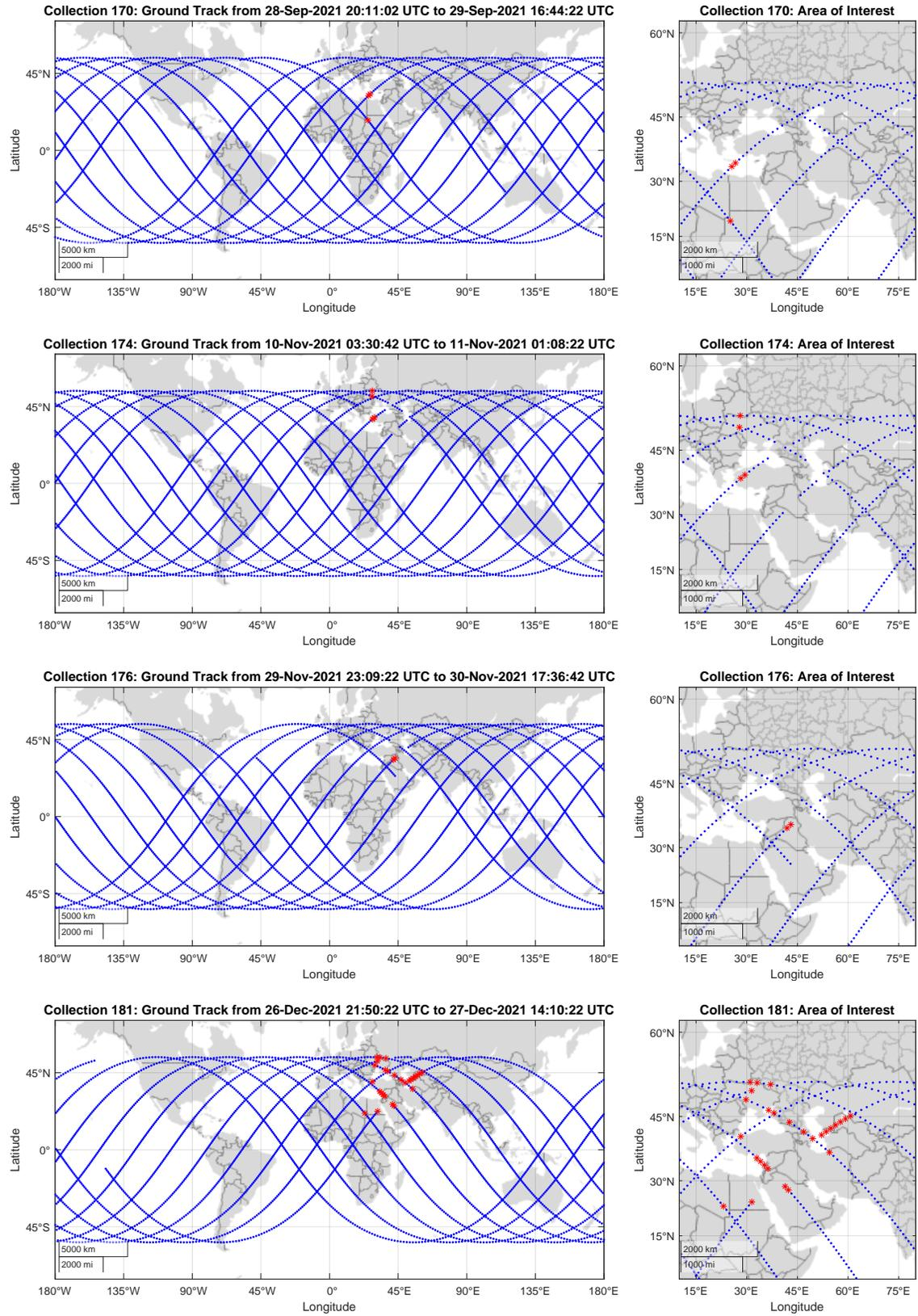
**Figure 3:** Bobcat-1's ground track during data collections with points of insufficient visibility to estimate GGTO marked in red.
