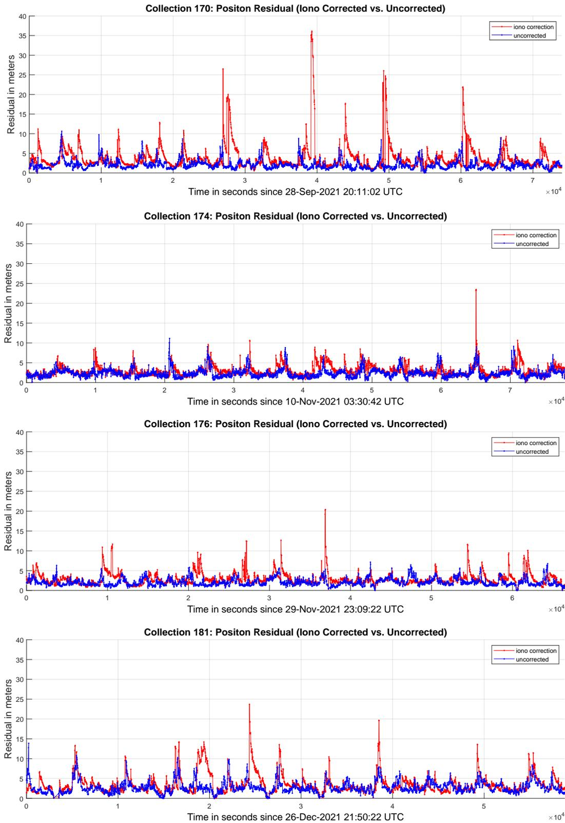
**Figure 4:** Comparing the position residuals with (red) and without (blue) ionospheric corrections applied for each data collection.
