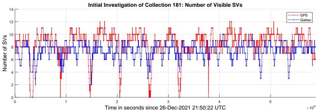
**Figure 2:** Number of visible SVs for GPS (red) and Galileo (blue) including data points with insufficient visibility.
