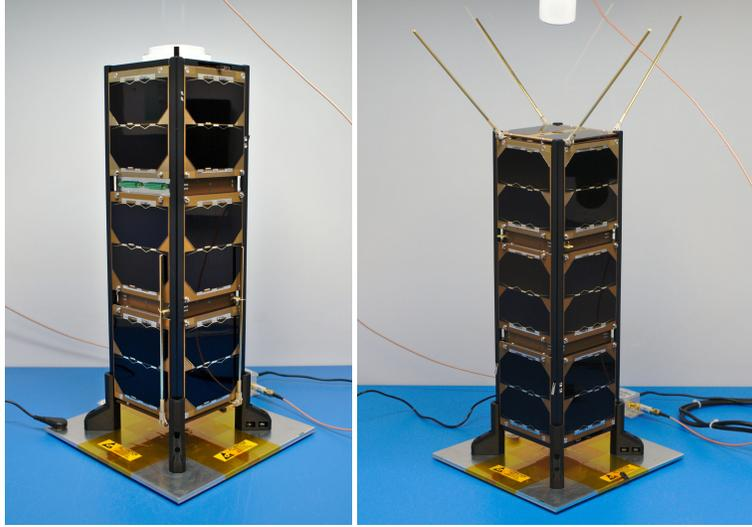
**Figure 1:** Bobcat-1, with communication antenna stowed (left) and deployed (right).
