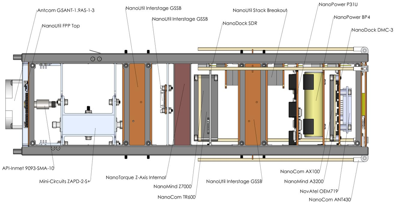
**Figure 2: Bobcat-1 cutaway view (solar panels not pictured)**
