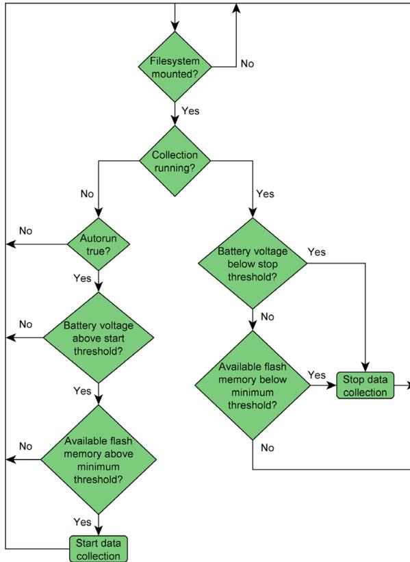
**Figure 4: Data collection control flowchart**
