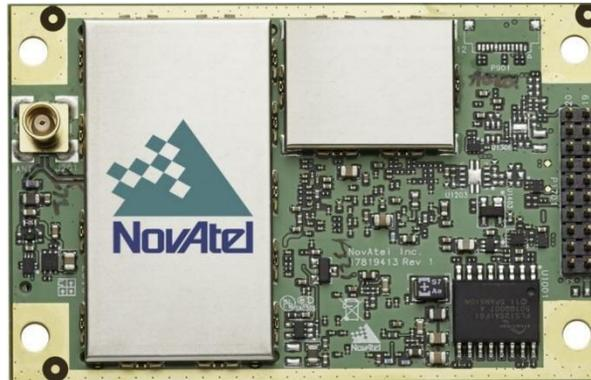
Figure 2. Novatel OEM719 GNSS receiver.
