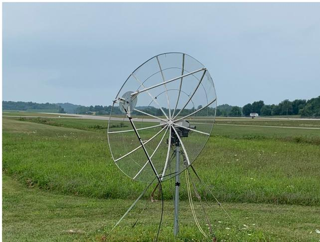
**Figure 2:** 1.9 m diameter parabolic dish located at the Ohio University Airport in Albany, OH
