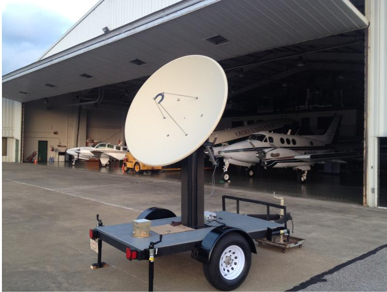
**Figure 2:**  $\sim 2$  m diameter solid dish on a mobile platform, to be used for the proposed experiment.
